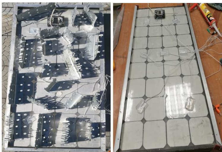
Fig. 5.24 (left) Modified panel with aluminum fins (right) referenced module
