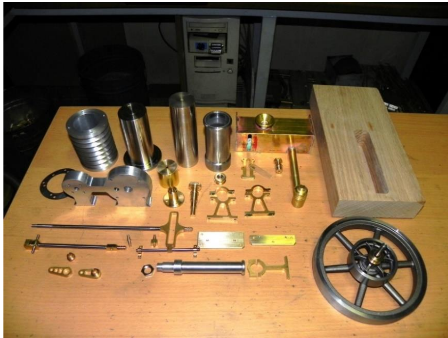
Figure 4-4: All parts of Gamma Stirling engine
