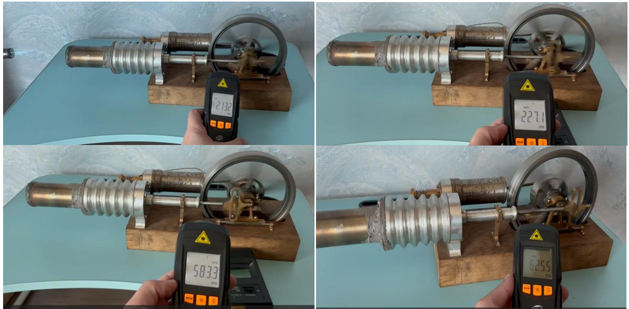
Figure 4-11: Gradual rise in rotational speed during the operating
