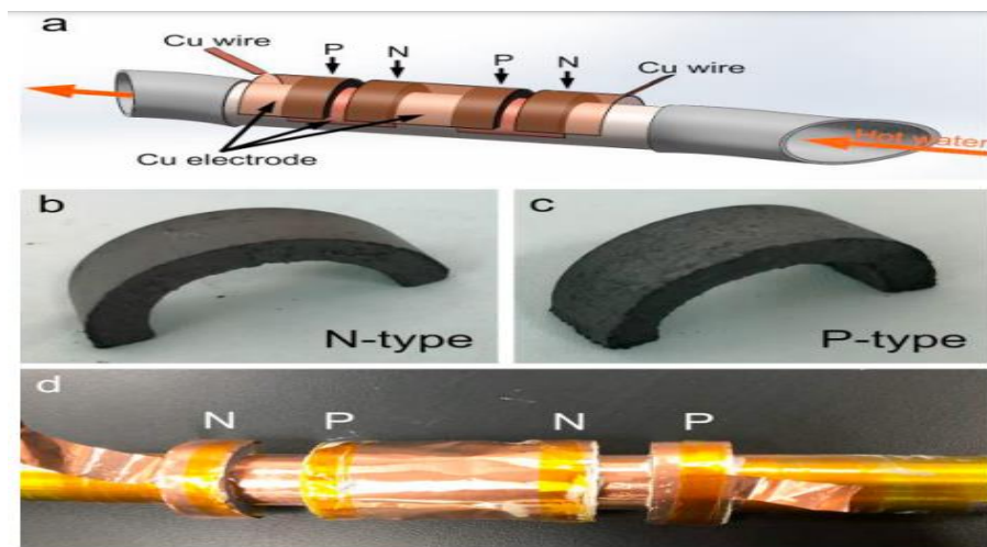
Figure 2-3 (a) Schematic of the TEG on a hot water pipe. (b) and (c) are the photographs of n and p-type half rings synthesized by compression molding, respectively. (d) Photograph of the TEG on a stainless steel pipe [56].
