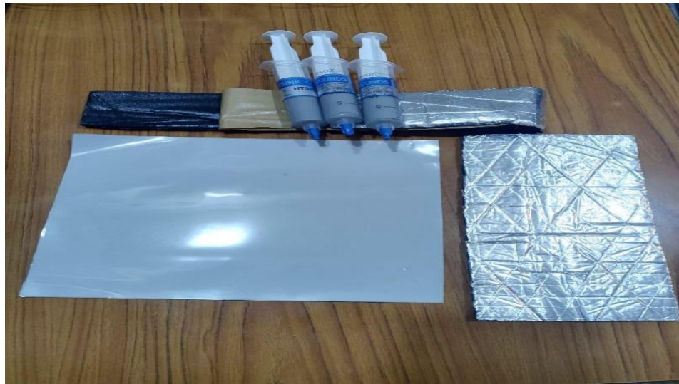
Figure 2-35 Thermal paste, arrays and insulators used in the panel
