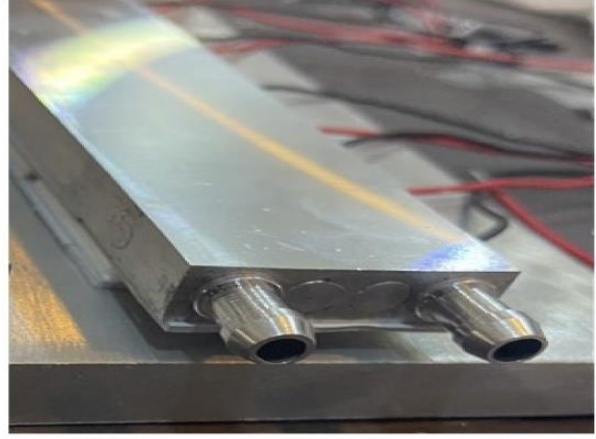
Figure 4-3 The practical configuration of the lower aluminum block with an M-shaped water channel
